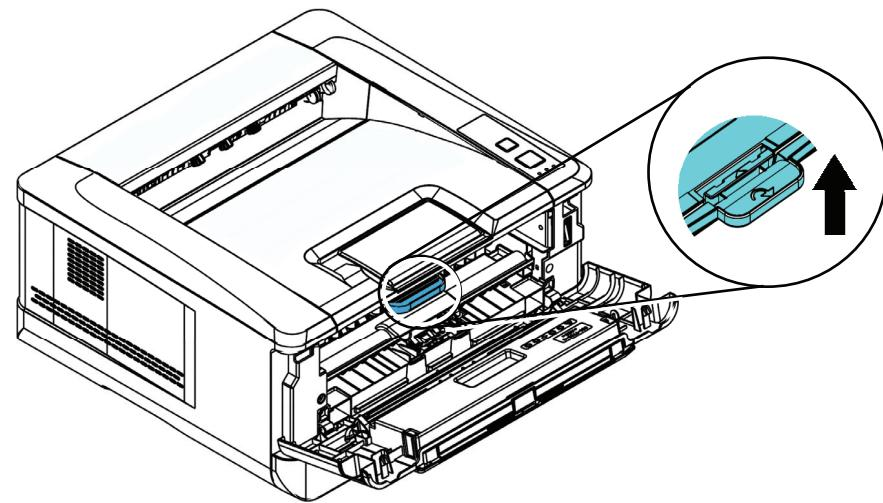
Step 3. Pull out the drum, and remove all the tapes on the drum.
