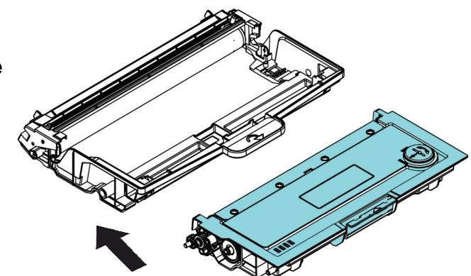
Step 5. Tilt the cartridge upward to slide in, push DOWN to snap in.
